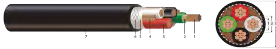
4/C CU 2000V EPDM/CPE Type W Industrial Grade Cable 90°C
